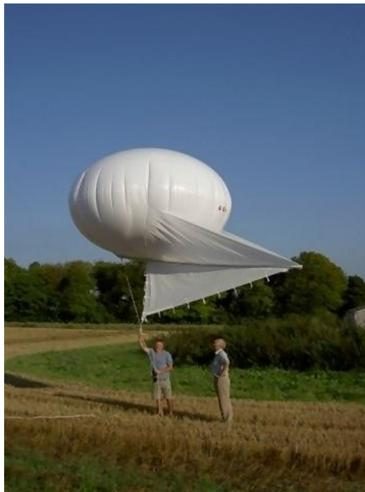
Picture 3. The combination of the balloon and the kite is the helikite [7]
