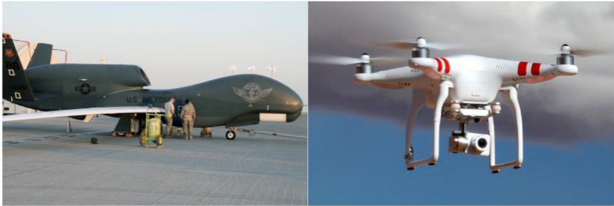
Picture 1. Fixed and rotary wing unmanned aerial vehicles [2][3]
