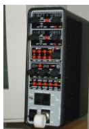
23. ábra. ACP aircraft control panel 10
