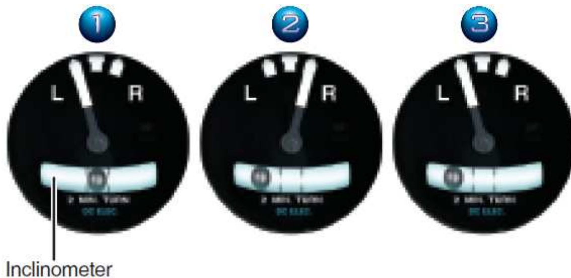
Figure 10. In a coordinated turn (instrument 1), the ball is centered. In a skid (instrument 2), the rate of turn is too great for the angle of bank, and the ball moves to the outside of the turn.
